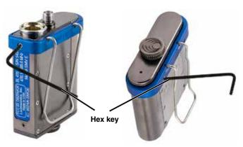
Align the set screws with the detents in the back cover, and tighten them with the supplied hex key until they are snug.
